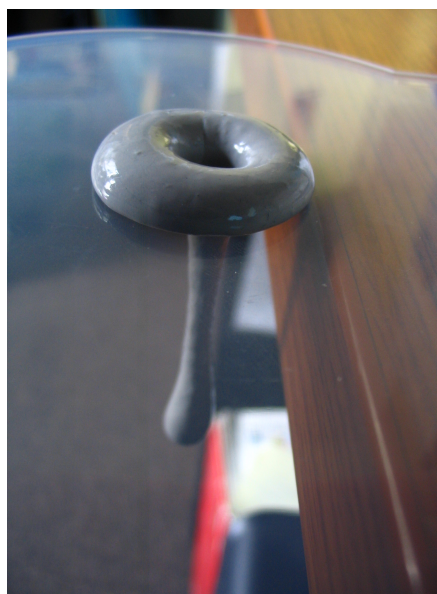
Figure 2: A lump of Silly Putty slowly dripping through a hole in a screen. 13
