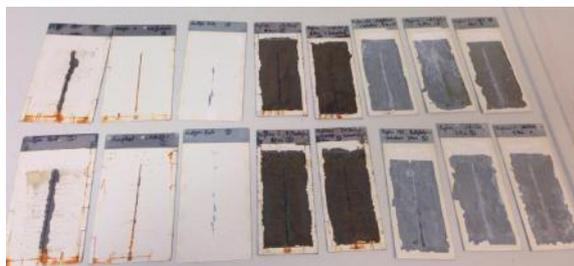
Figure 9: Pictures of the Treated Samples After 215 Hours SST. Left to Right: Steel, Phosphate Steel, Zinc, PA/Molybdate/Leveling Agent on Steel, PA/Molybdate on Zinc, and PA/Tungstate on Zinc.
